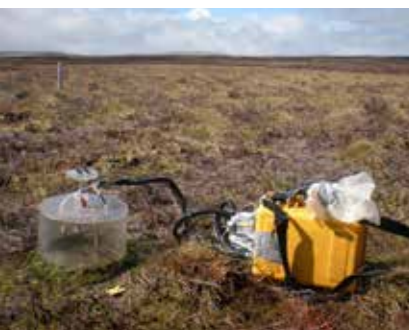
Carbon flux monitoring over recently managed ground
